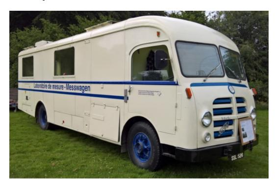
This example, owned by a local collector of what he called "his toys", was built in 1954, initially for the Swiss Army as a mobile X-ray clinic able to travel to avalanche sites and the like. It has a six cylinder, 8.6 litre diesel engine, giving around 115 bhp and a comfortable maximum speed of 40 mph, though with the ability to climb as well, if a little slowly. Some one asked if it would do 70 mph, downhill? A brave idea, I suggest.
