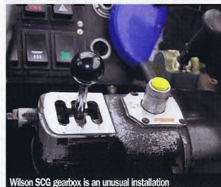
Wilson SCG gearbox is an unusual installation
