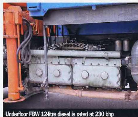
Underfloor FBW 12-litre diesel is rated at 230 bhp
