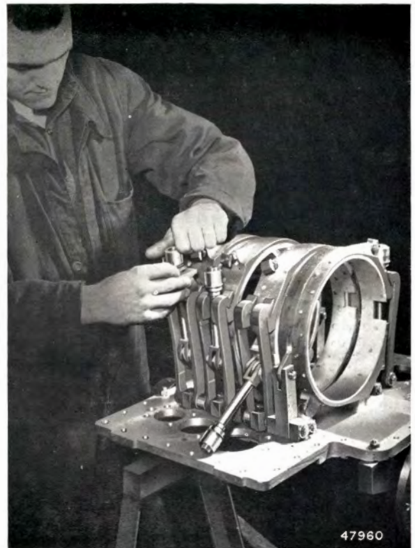
FIG. 22. FITTING THE AUTOMATIC ADJUSTERS
