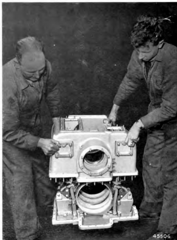
FIG. 27. FITTING THE GEAR CASE TO THE BOTTOM COVER ASSEMBLY
