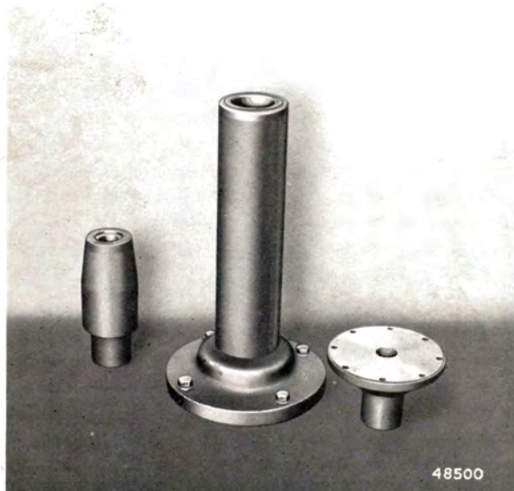
FIG. 14. ASSEMBLY STAND AND ADAPTERS
