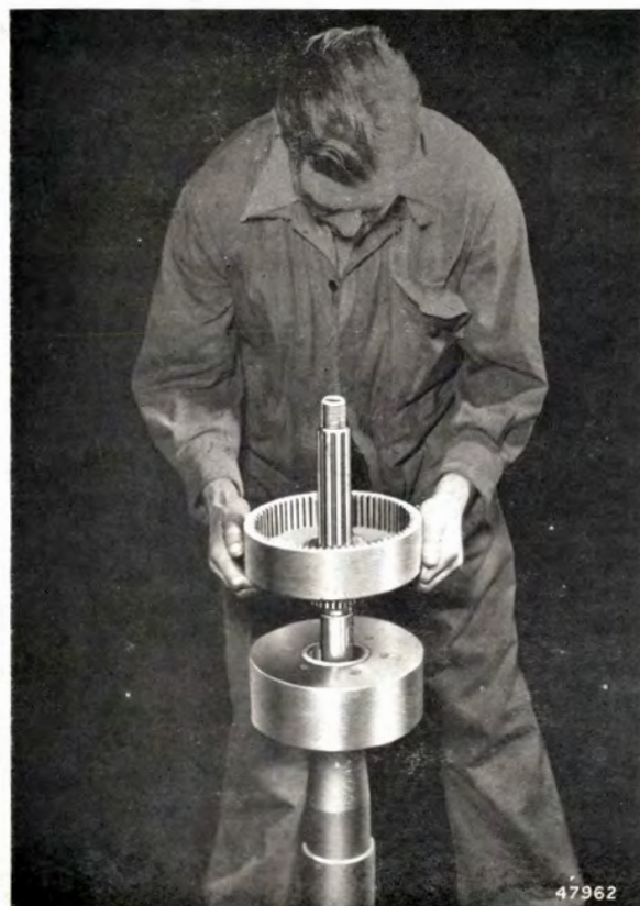
FIG. 36. FITTING THE 3rd SPEED BRAKE DRUM
