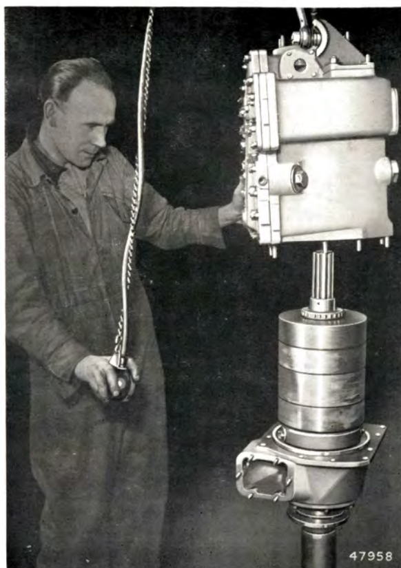
FIG. 40. FITTING GEAR CASE TO RUNNING GEAR
