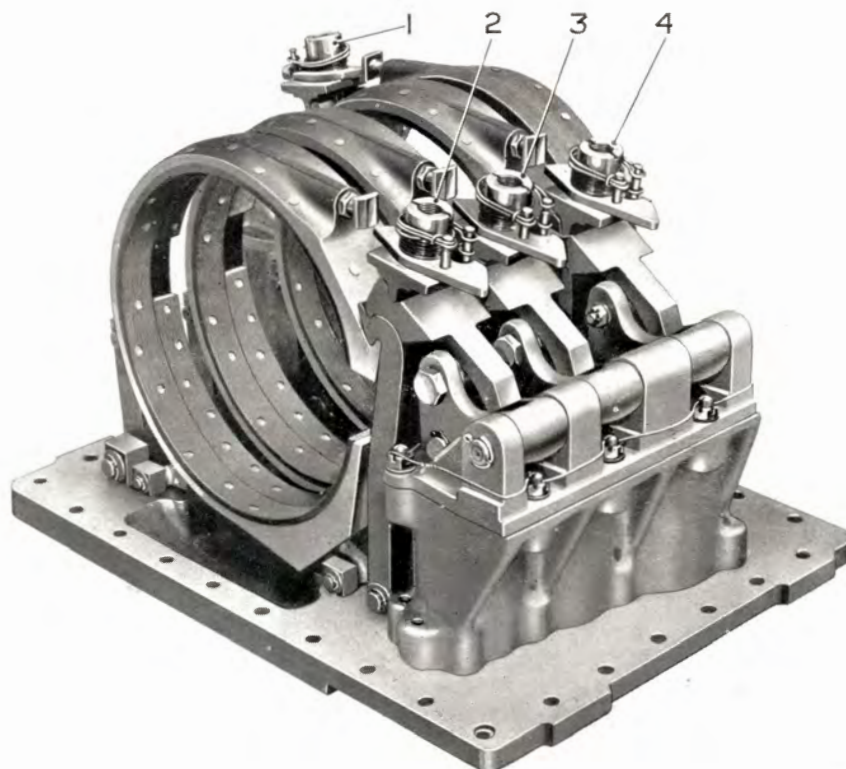
FIG. 25. THE BOTTOM COVER AND BRAKE BAND ASSEMBLY
