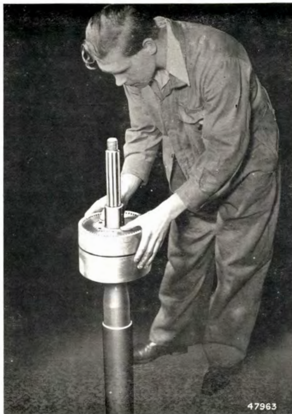
FIG. 37. FITTING THE TOP SPEED CLUTCH PLATES
